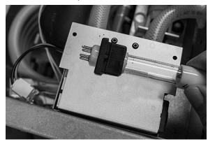
6. Align slot on LuminIce® and notch on retainer and install replacement bulb in LuminIce®.
