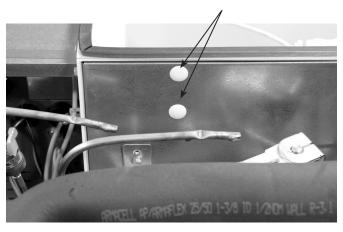
3. Remove bracket from ice machine and assemble LuminIce®, tubing and secure with hose clamps.
