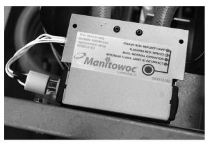
4. Push bulb with finger and pull with other hand toward the rear of the ice machine until bulb is free.
