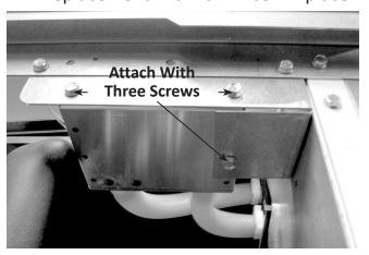
5. Refer to picture and install LuminIce® hoses, wire clip and secure wires to clip.
