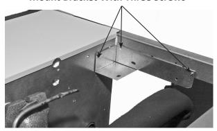
4. Assemble LuminIce® to bracket with three screws provided. The bulb and bulb wiring must face toward the rear of the ice machine to allow bulb replacement with LuminIce® in place.
