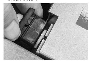
7. Insert bulb until it seats in the retainer stop on the opposite end.
