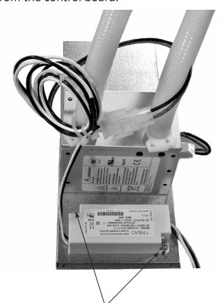
Mount LuminIce® And Power Supply To Bracket Indigo® Models Only
