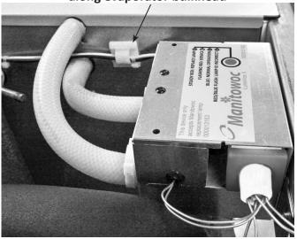
6. Install the notched evaporator dust cover from kit.
