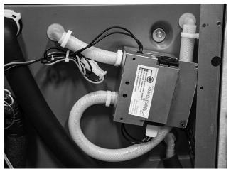
5. Mount LuminIce® to ice machine with 2 screws.
