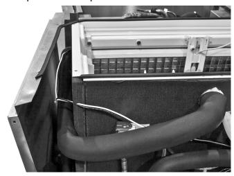
9. Install the evaporator dust cover and test run the ice machine and LuminIce®. The LuminIce® is energized whenever power is applied to the ice machine. A noticeable draft will be emitted from the upper hose adapter during operation.
