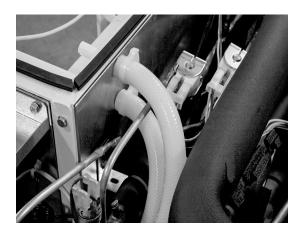
5. Install the evaporator dust cover and test run the ice machine and LuminIce®. The LuminIce® is energized whenever power is applied to the ice machine.
