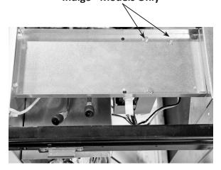
4. Assemble bracket to ice machine.
