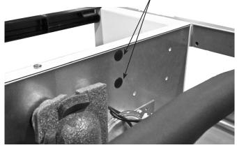
3. Assemble bracket to left-hand top rail with three provided screws.
