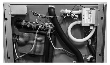
8. Reinstall bin, wire connectors and all panels, then test run. A noticeable draft will be emitted from the upper hose adapter during operation.
