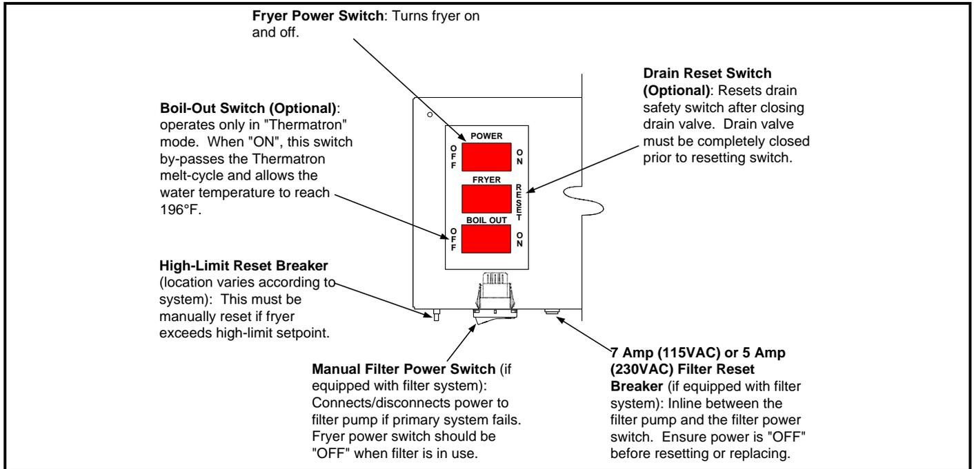
**FRYER POWER SWITCH** – This switch turns the fryer on and off. When the power switch is in the "ON" position, the indicator light will be lit when calling for heat.
