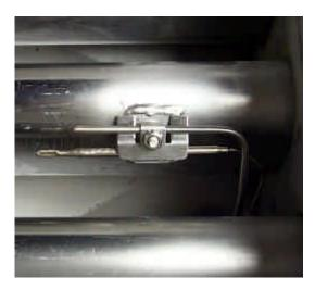
Typical high-limit/sensor probe locations and mounting hardware.
