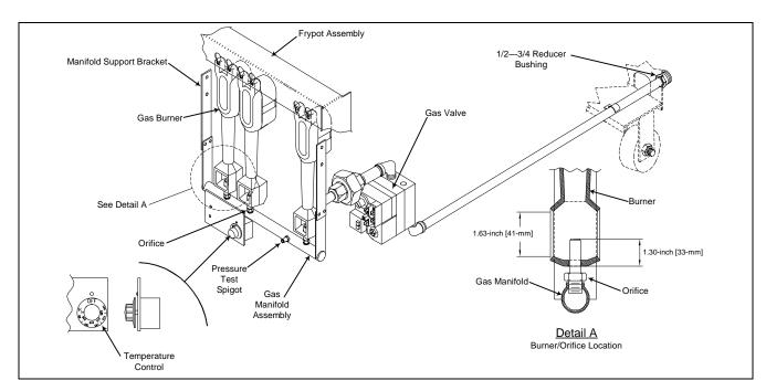
Typical gas valve, burner and orifice locations
